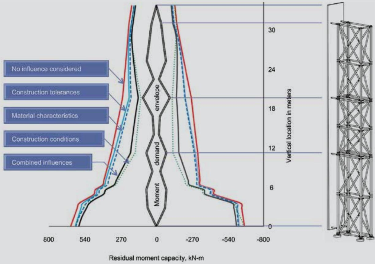
**Figure 5.** Variations in individual material and geometric parameters can reduce the residual cracking moment capacity of a shored wall panel. Due to internal stresses, the cracking moment capacity can potentially be reduced by up to 50%. Note: 1 m = 3.28 ft; 1 kN = 0.225 kip .
