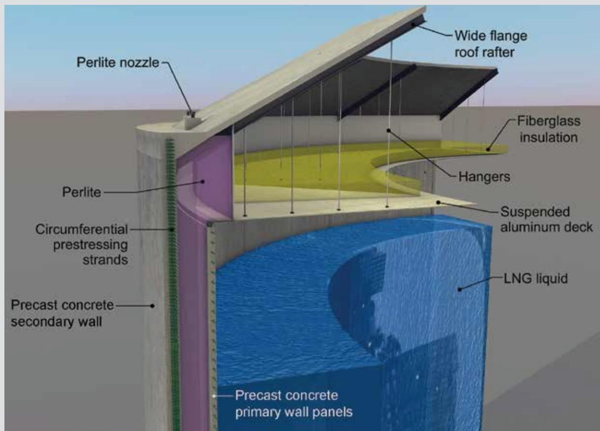
**Figure 4.** Cutaway section at the top of the composite concrete cryogenic LNG storage system. The concrete roof is part of the secondary containment and the suspended deck supports the thermal insulation over the stored LNG in the primary containment. Figure courtesy of BergerABAM. Note: LNG = liquefied natural gas.
