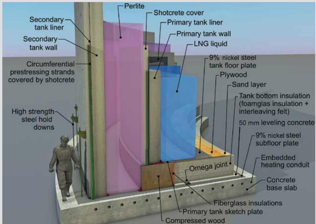
**Figure 3.** Cutaway section at the base of the composite concrete cryogenic LNG storage system. Precast concrete walls are used for both the primary and secondary containment. The annular space between the primary and secondary containment walls is filled with loose perlite insulation. Figure courtesy of BergerABAM. Note: LNG = liquefied natural gas. 1 mm = 0.0394 in.
