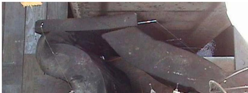
**Figure 8. Fender of test bed failing long-term test in first tide cycle.**
