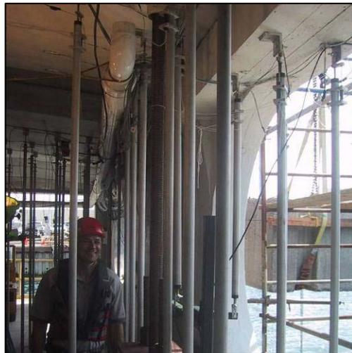
**Figure 6. Upper deck capacity test on test bed.**
