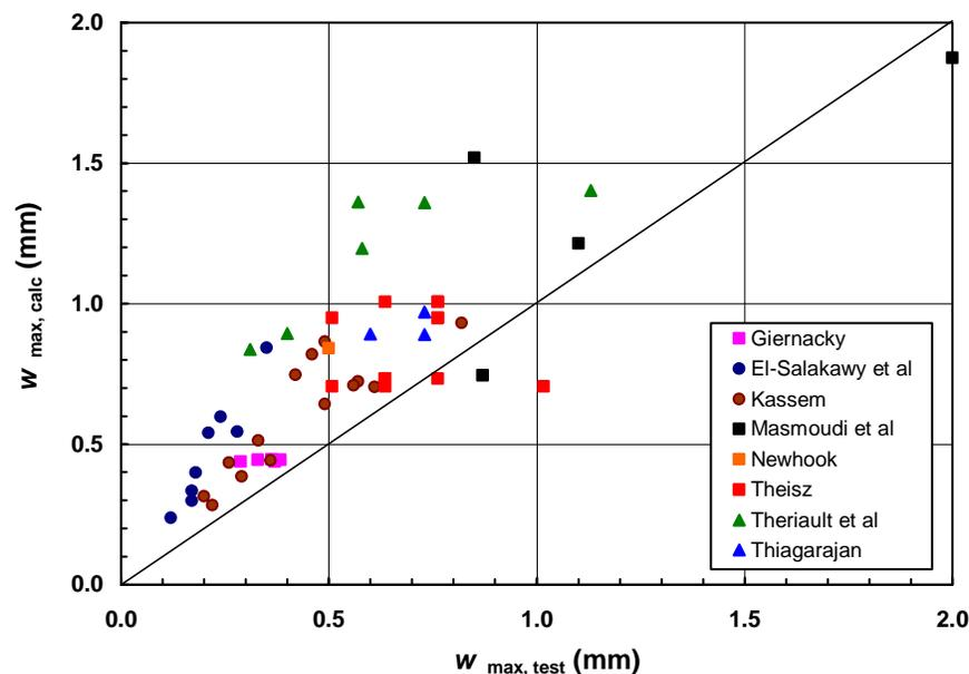
Fig. 2 Comparison Between Eq. (1) Predictions and Experimental Evidence.
