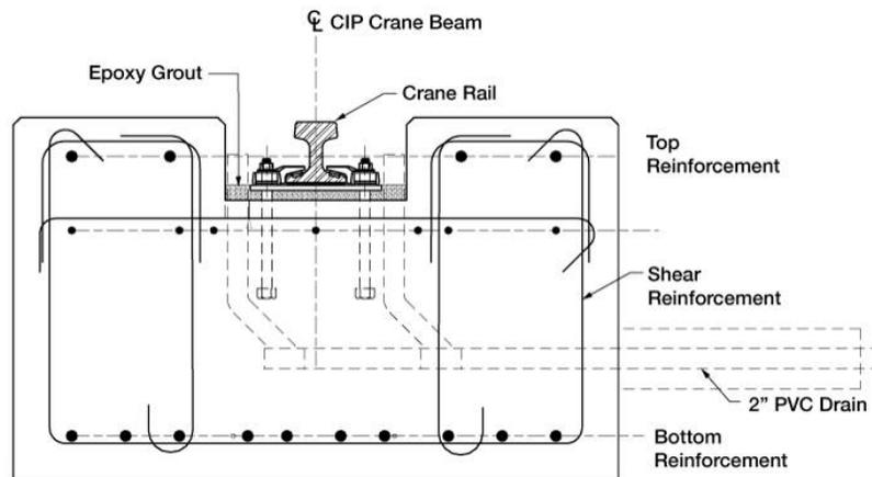
**Figure 6. Typical section of a crane rail foundation.**
