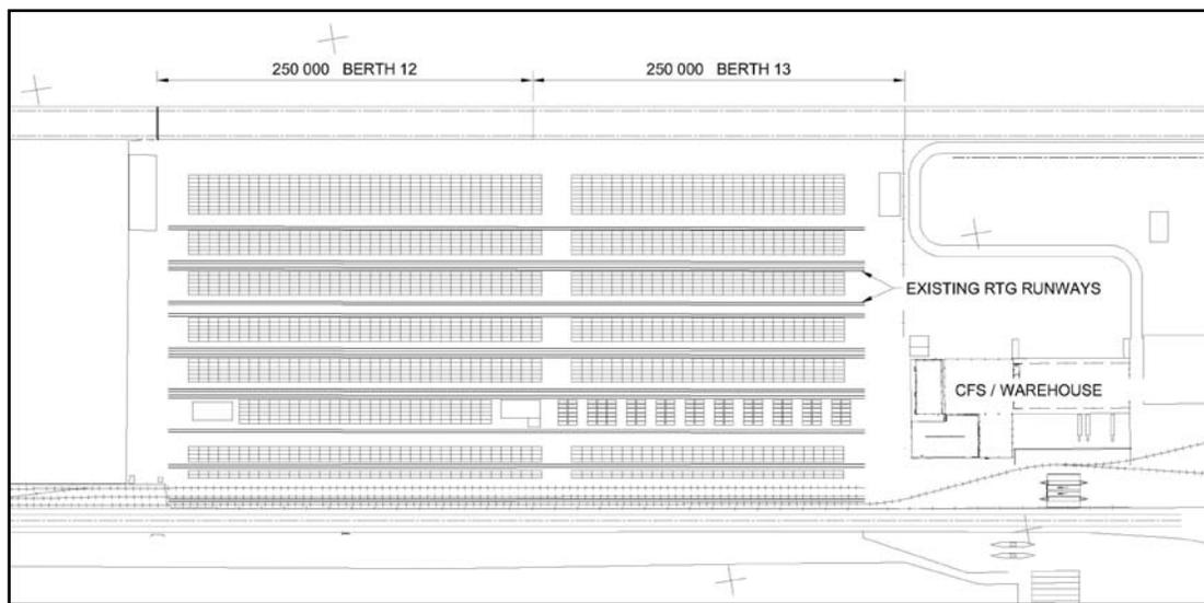
**Figure 2. Berths 12 and 13 container yard layout.**
