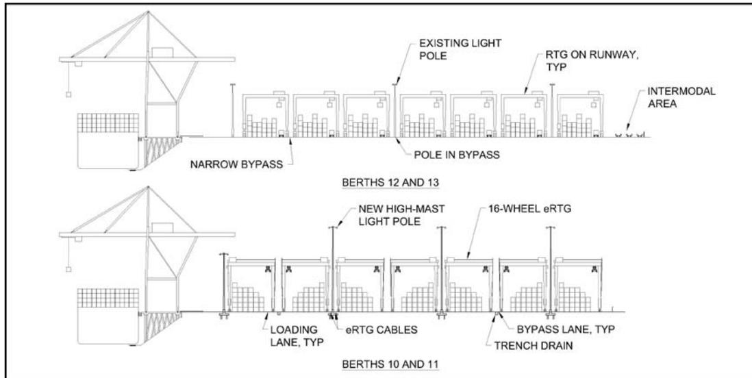
**Figure 4. Comparison of berths container yard sections.**
