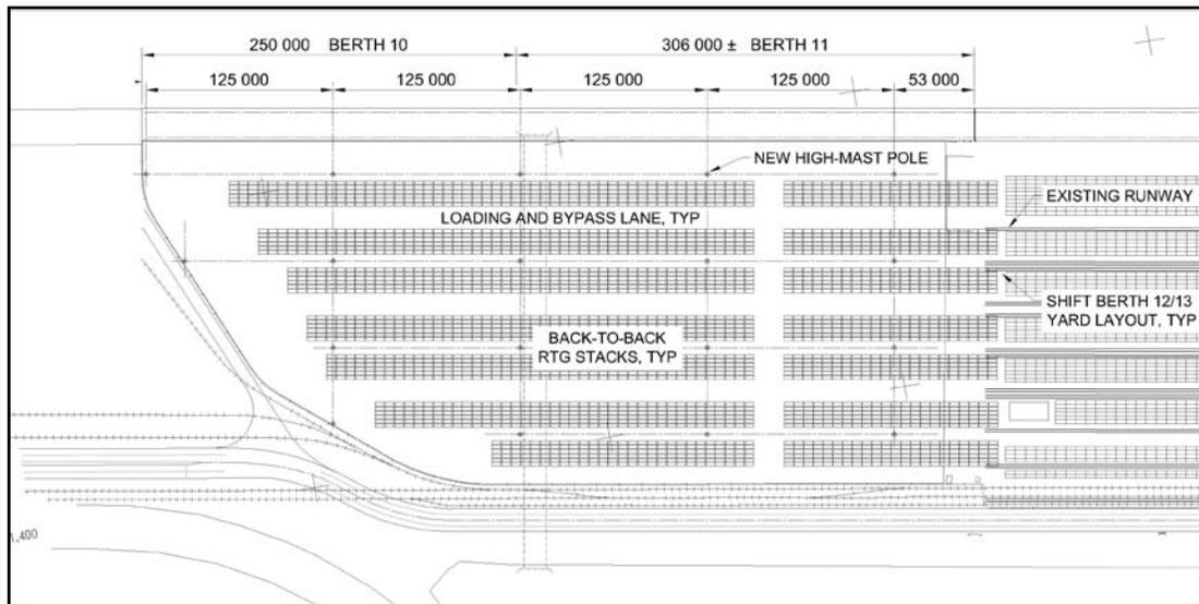
**Figure 3. Berths 10 and 11 container yard layout.**
