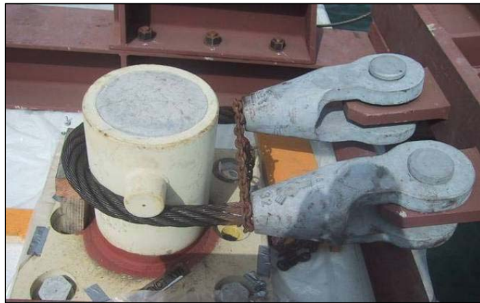
Figure 10. Bollard test on test bed.
