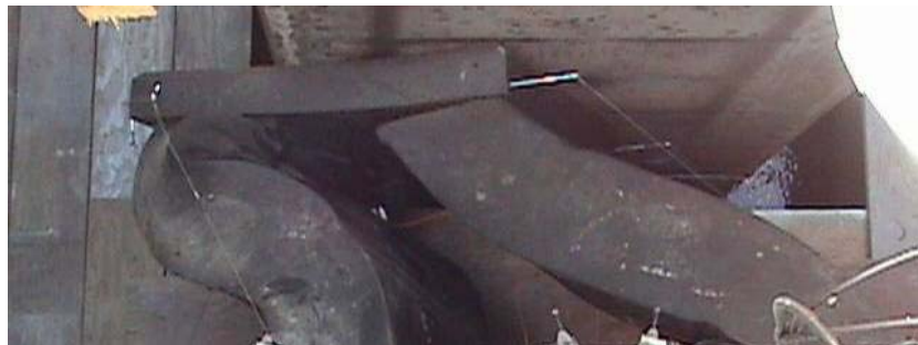
Figure 8. Fender of test bed failing long-term test in first tide cycle.
