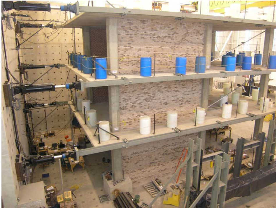
Figure 2. Test Structure with Infill Walls
