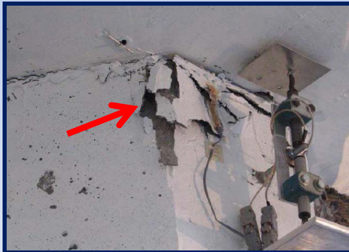
Pile Crushing \mu_{\Delta} = 6 (3.4% drift)
