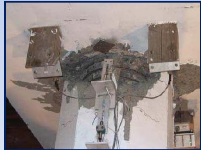
Test Ended \mu_{\Delta} = 16 (12.9% drift)
