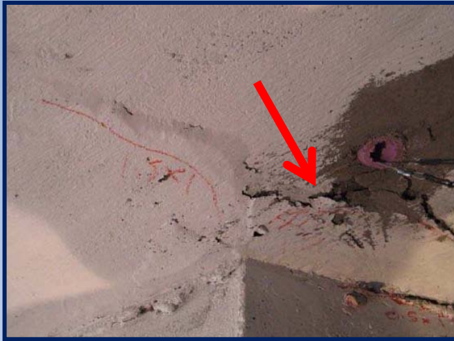
Slab Prying \mu_{\Delta} = 1.5 (1.2% drift)
