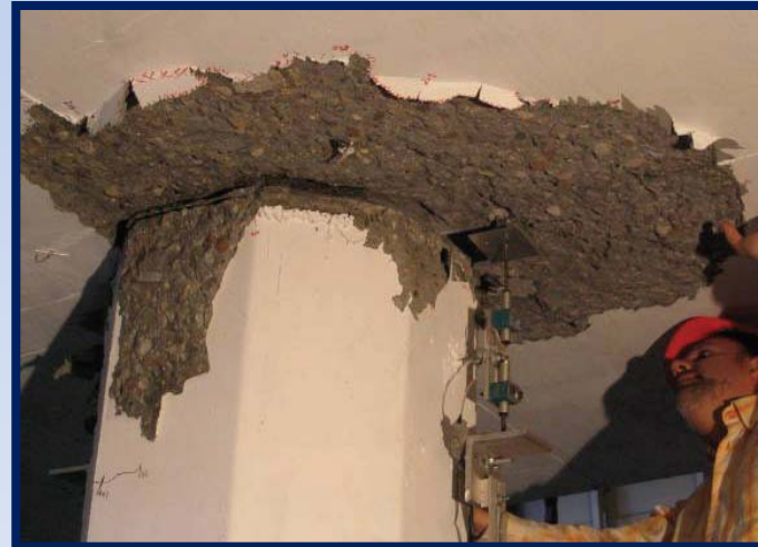
Test Ended \mu_{\Delta} = 18 (10% drift)
