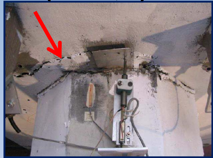
Deck Crushing \mu_{\Delta} = 2 (1.6% drift)
