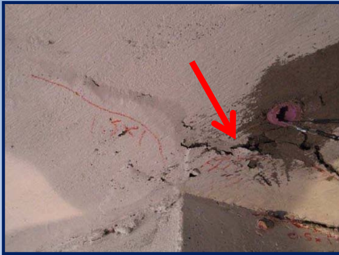
Slab Prying \mu_{\Delta} = 1.5 (1.2% drift)
