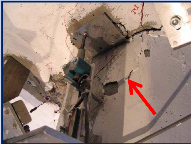
Pile Crushing \mu_{\Delta} = 3 (2.4% drift)
